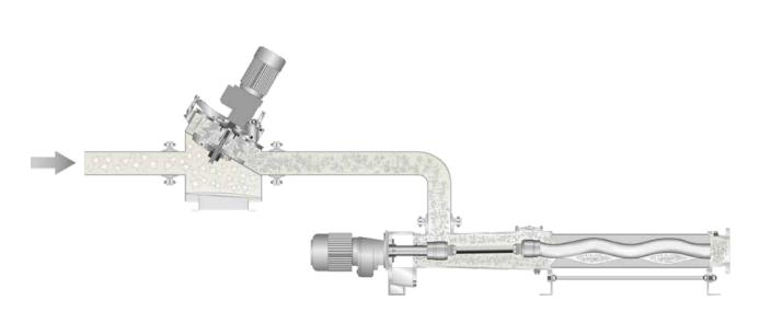
NEMO® BY progressing cavity pump with a cutting plate macerator M-Ovas®
