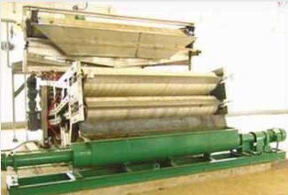
NEMO® Sludge cake pump with 2 meter hopper design underneath a belt filter press conveying sludge 120 ft (37 m) to the drying plant. Solids content approximately 20%, flow-rate of 26 gpm (6 m<sup>3</sup>/hr) at 120 psi (8 bar) discharge pressure.
