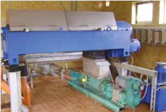
NEMO® Sludge cake pump being utilized underneath a centrifuge to convey dewatered sludge over 137 ft (42 m) to transport truck. Solids content approximately 18%, flow rate of 2–3 gpm (.45–.7 m<sup>3</sup>/hr) at 30 psi (2 bar) discharge pressure.
