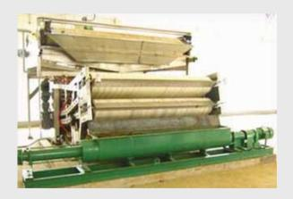
NEMO<sup>®</sup> Sludge cake pump with 2 meter hopper design underneath a belt filter press conveying sludge 120 ft (37 m) to the drying plant. Solids content approximately 20%, flowrate of 26 gpm (6 m<sup>3</sup>/hr) at 120 psi (8 bar) discharge pressure.
