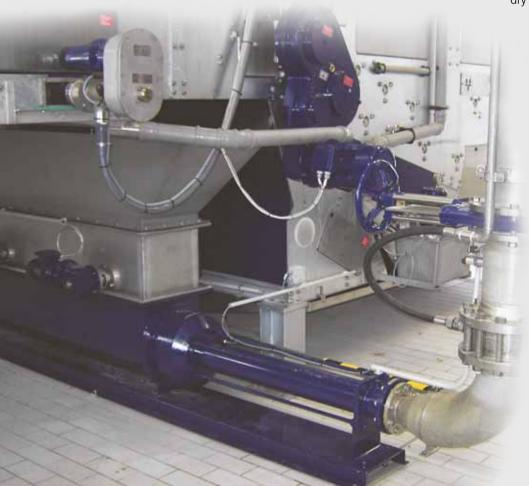
NEMO® Sludge Cake Pump with customized 1.5 meter hopper pumping 20 - 22% dewatered sludge from a belt filter press to a drying plant 110 ft. (34 m) away. Pump employs dual aBP-Module (Asynchronous Bridge Preventing Module) and STP stator run dry protection system.
